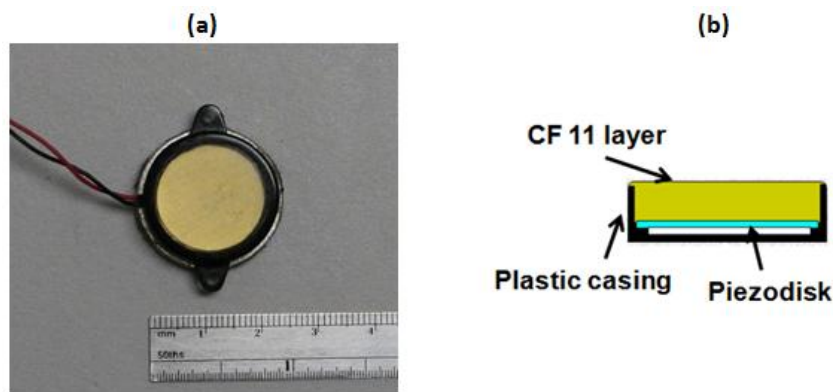
Figure 5.7 (a) Silicone gel coupled piezodisk sensor (b) schematic diagram of the sensor.
