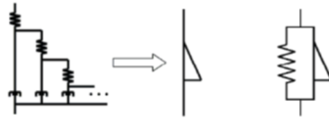
Figure 2.1 A tree arrangement of springs and dashpots (left) resulting in a fractional order element, called a springpot (middle). Schematic representation of a fractional order Voigt model (right); the dashpot is replaced with a springpot.
