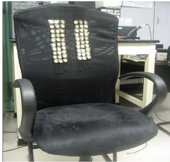
Figure 5.10 Piezodisk sensors imbedded on a chair.
